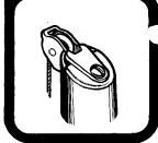
SHROUDS are attached to lightweight, low windage tangs in stainless steel. Double tangs are fitted where a trapeze is to be used. Forestay attachment is integral with the jib halyard sheave cage which is welded into the mast. This sheave cage is unique in that it passes through the mast angled down in the fore and aft vertical plane. This facili-
