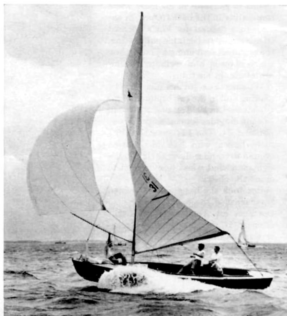
FASTEST of the large planing classes, 24-foot Raven, needs more wind to plane than smaller hulls, has more speed than conventional boats of similar size. Only comparable boats as fast are the wide, flat-bottom scows, popular for lake sailing in midwestern U.S.
