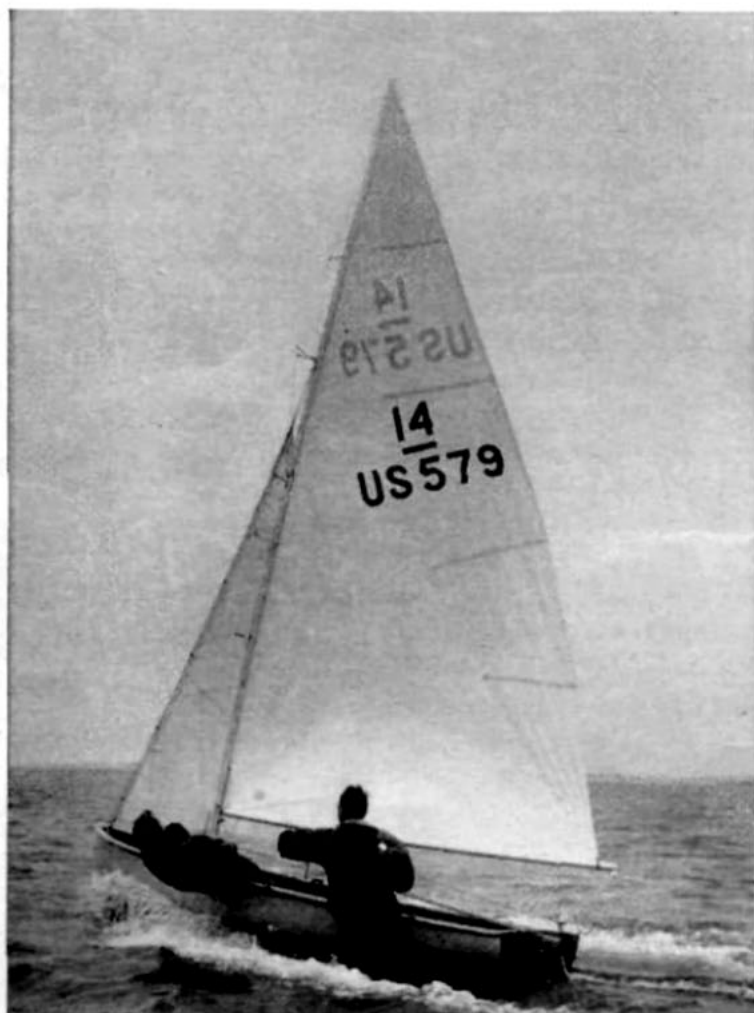
FIRST small planing hull, the International 14 was prototype for more recent planing classes. For racers who prefer rugged sailing, like North American Sailing Champion George O'Day ( at helm below ), this is still a favorite type.
