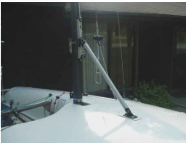
Photo 6: Mast Ram Mounted
