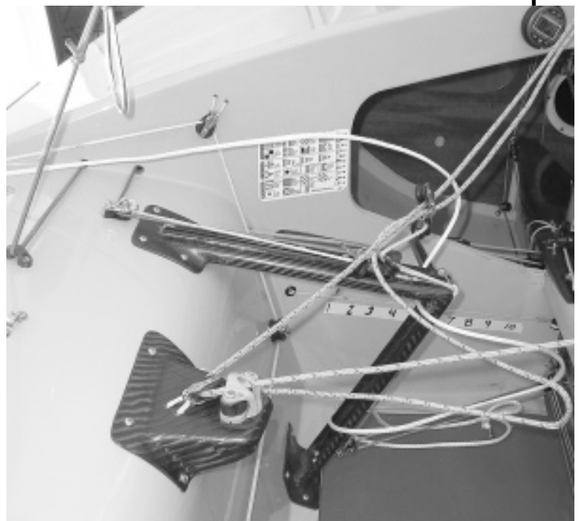
2:1 jib sheets, with the capacity to sheet inboard via custom carbon jib lead system.
