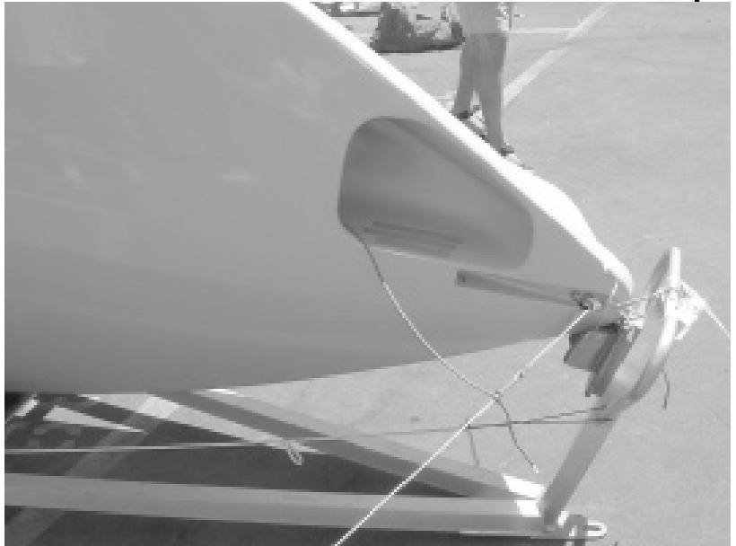
Offset spinnaker launcher tube on USA 8854 allows for a forward jib tack position.
