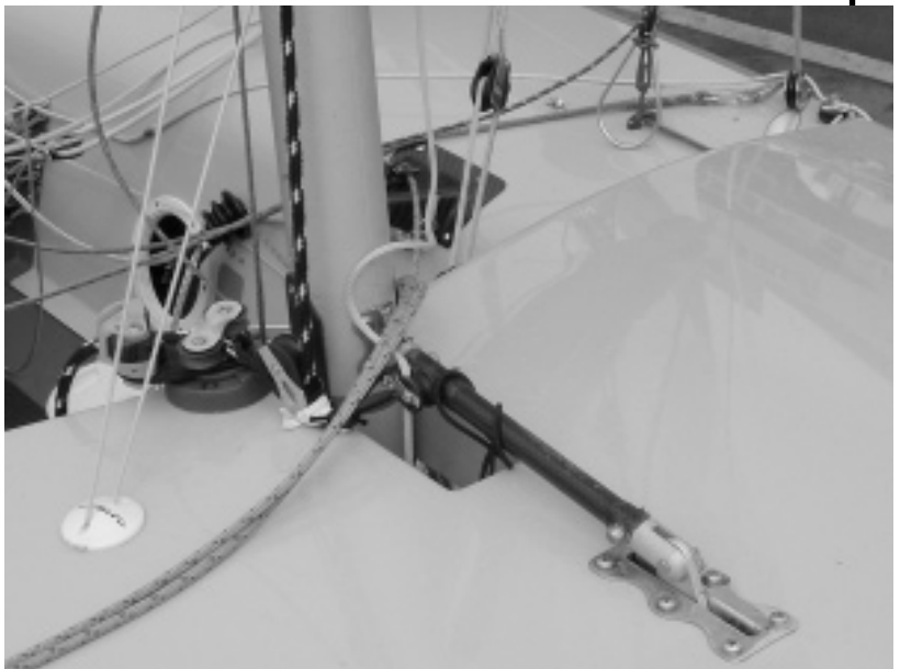
A deck-level mast pusher allows for a "proper" foreguy unobstructed by a diagonal ram strut.
