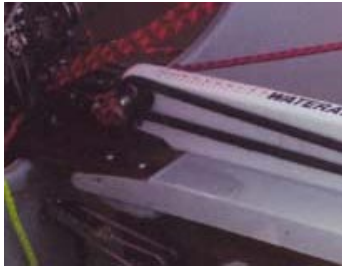
Two boards: Standard Waterat board (left) sports snug fit. High-aspect board (right) sits taller above trunk.
