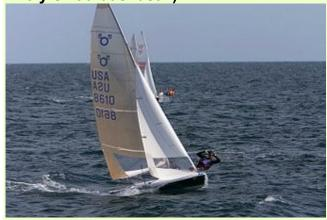
It is a 16.5 foot (or 5.05 meter) centerboard racing boat that is designed to be raced with two people. The forward crew is sailing from a **trapeze** and the driver is hiking on straps.
